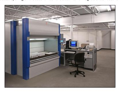
If a requested part is located in bin storage, a clerk on the second-floor mezzanine delivers it to the first-floor parts department using an open tray in the Shuttle XP VLM, eliminating the need for additional personnel to move parts between floors manually.
