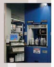
"During the setup of each job, the software will confirm the stock of each item being used. It continually tracks the quantity of each sub-component and allows for the "pre-plenishment" of machine located SMT feeders. This is one of the keys to our efficiency and reduced downtime."
