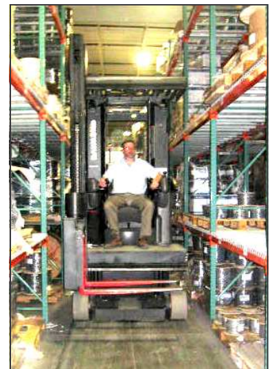
Raymond's Swing Reach truck made the narrow aisle pallet handling possible.
