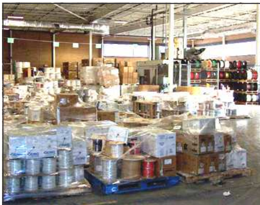
Existing floor and rack storage areas were replaced with more efficient narrow aisle racks and wire guided lift trucks. The design allowed Tappan to regain 9,000 SF for manufacturing .
