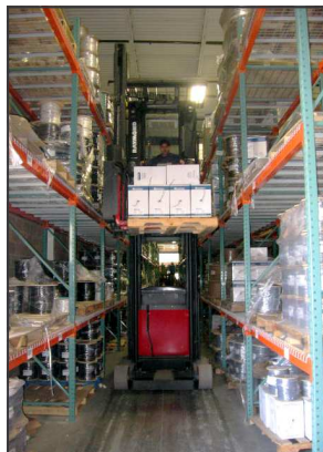
Existing floor and rack storage areas were replaced with more efficient narrow aisle racks and wire guided lift trucks. The design allowed Tappan to regain 9,000 SF for manufacturing .
