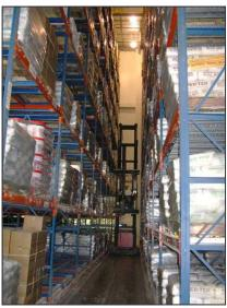
Raymond's Swing Reach truck made the narrow aisle pallet handling possible for increased operator productivity.
