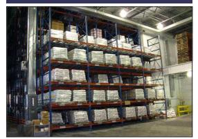
With the deep pallet flow through rack, the 40 fastest moving SKUs are readily available from the other side.
