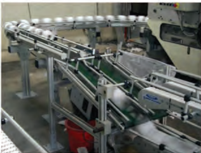
Paper converting line with diverter
