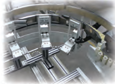
Automated side guide installed at bend section
