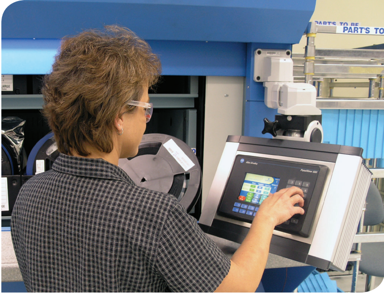
MicroLogix 1500 controllers including a Panel View operator interface allow the vertical carousel to present the correct reel with a push of a button.
