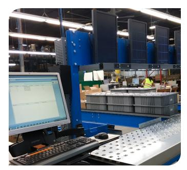
Display monitors at the batch station show the operator the exact tote cell to place the item, allowing fulfilling 120 orders in a single batch.
