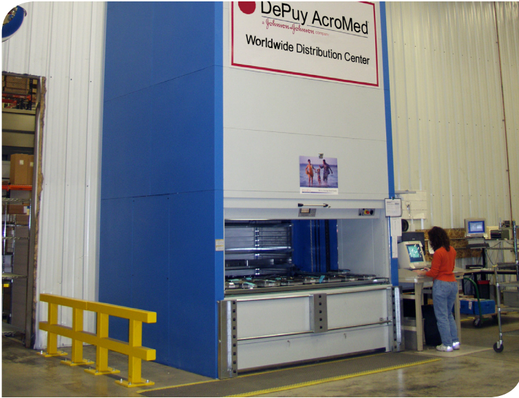
Up to 500 transactions a day are made from the Shuttle VLM which queues up to 2000 kits.
