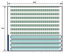
575 sections of shelving has the same storage capacity as four 79.1' long horizontals carousels.
