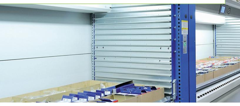
The Kardex Remstar Shuttle<sup>®</sup> Vertical Lift Module (VLM) has been designed to meet a broad range of storage and retrieval applications in manufacturing, distribution, retail and warehouse operations. The combination of storage density, flexibility, efficiently and security makes it an ideal storage solution for most every application!
