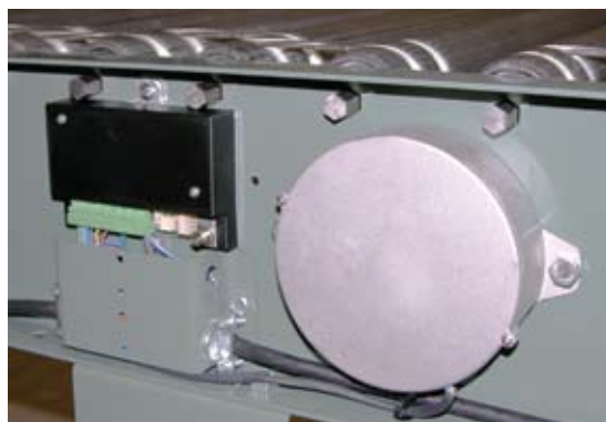
Rollers are powered by 24 VDC motors. The rollers are driven from the motor with o-rings.
