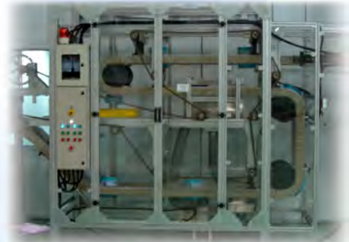
Gripper conveyor with blower attached to remove dust from products.
