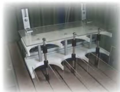
To avoid can from toppled when transferring from one conveyor line to another
