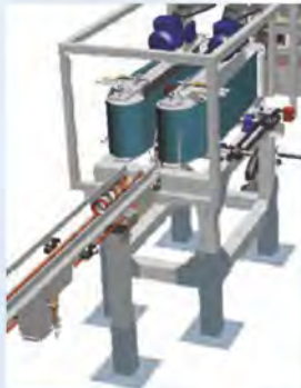
Composite can from polycord conveyor traveling to Uppender
