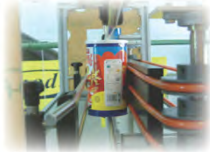
Stainless steel rod is use to maintain orientation.
