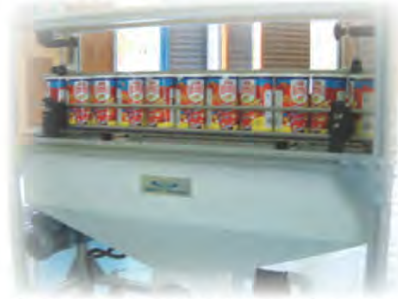
Product is transported to another machine while being dust blowing.
