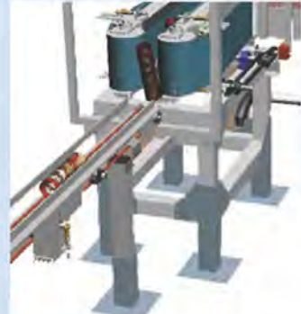
Composite can changes orientation at Uppender
