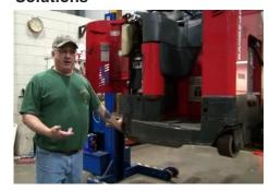
An increasingly popular solution among maintenance crews is the TechMate. Abel Womack has been working closely with AG for years and dropped by to give a full demonstration of the battery-operated service lift. They provided training for AG's primary users so they'd be fully comfortable loading and securing varying trucks using the hydraulic lift with a locking mechanism.
