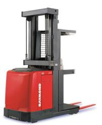
24 Volt 3000 lb. capacity 95" collapsed height 204" elevated height
