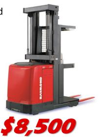
24 Volt 3000 lb. capacity 95" collapsed height 204" elevated height
