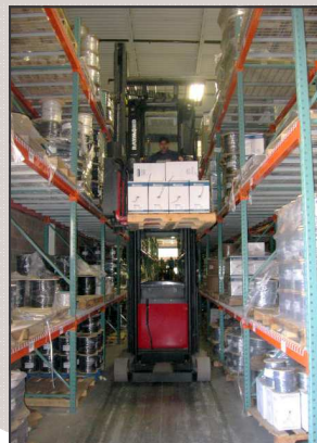
Existing floor and rack storage areas were replaced with more efficient narrow aisle racks and wire guided lift trucks. The design allowed Tappan to regain space for manufacturing purposes.
