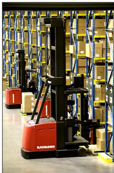
Left: Operator picking in a very narrow aisle. Right: Operators using Orderpicker trucks to pick or place product.
