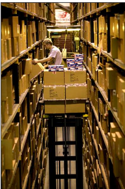
Left: Operator picking in a very narrow aisle. Right: Operators using Orderpicker trucks to pick or place product.
